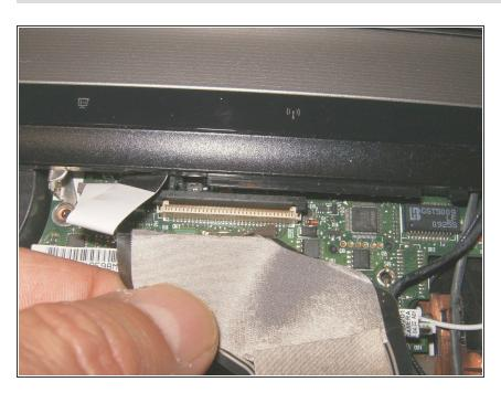
Here is the keyboard ribbon cable seated in the zero insertion force (Zif) connector. The keyboard is now separated and can now be removed. To reassemble your device, follow these instructions in reverse order.
