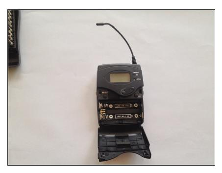
Turn off the transmitter and take out the batteries.
