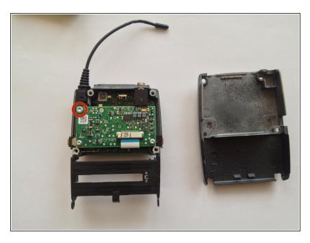
Remove the back cover and remove one more torx screw on the upper left corner.
