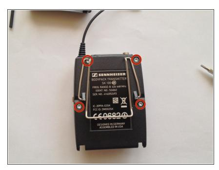
Remove the 4 torx screws on the back.
