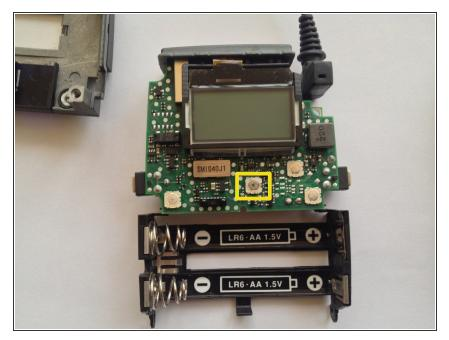
Carefully remove the front cover and locate the tactile switch that's giving you a hard time.
