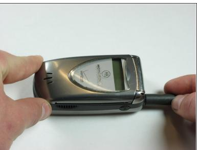
Detach antennae by unscrewing in a counterclockwise fashion.
