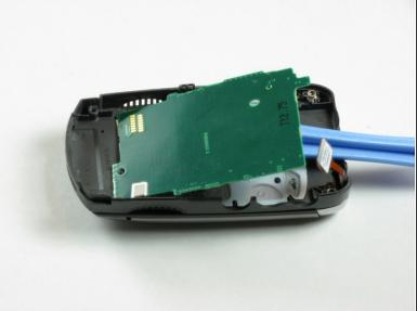
Insert spudger under button board and gently lift, set aside.
