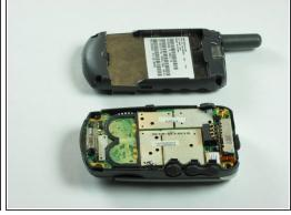
Use a spudger to gently pry off back chassis. Wedge the spudger in crevice between back panel and phone and lift.
