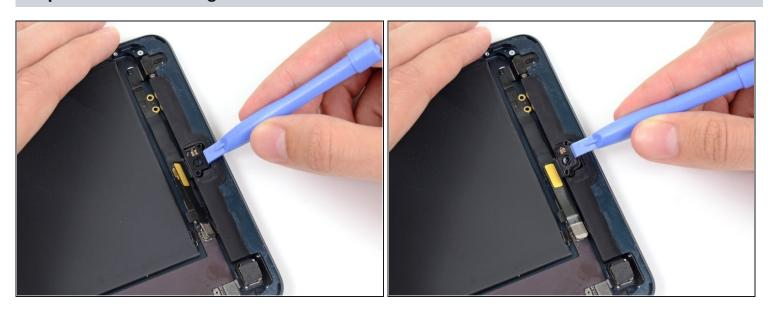
Use a plastic opening tool to gently pry the front-facing camera forward, separating it from the adhesive securing to the rear case.
