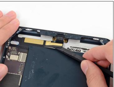
• Slide the flat end of a spudger underneath the Lightning port cable, freeing it from the adhesive securing it to the rear case.
