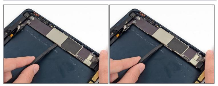
• Insert the flat end of a spudger underneath the center of the logic board. Slowly pry to free the section from adhesive.
