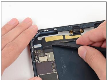
• Continue to carefully slide the spudger under the Lightning port cable nearest the logic board.
