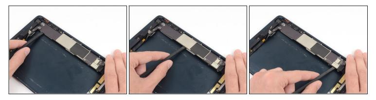
• Insert the spudger further under the logic board and slide along its length to detach the last of the adhesive.
