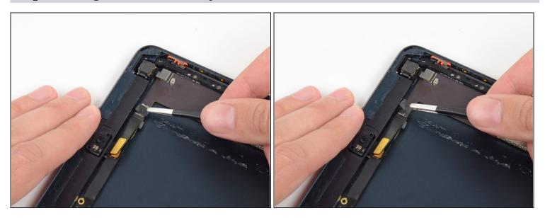
• Use tweezers to peel up and remove the small piece of tape covering the front-facing camera cable connector.
