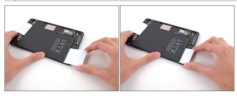
• Slowly push the card in further, breaking more of the adhesive between the battery and the rear case.
