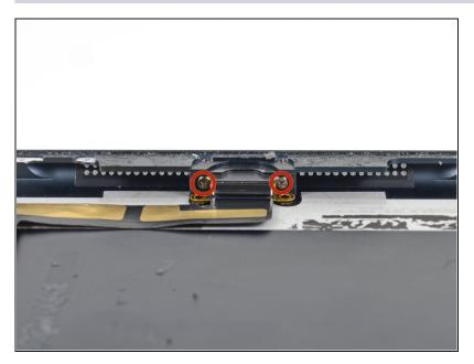
Remove two 2.8 mm Phillips #00 screws from the base of the Lightning connector.
