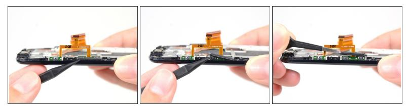
• Use the tip of a spudger to push the volume rocker button cover out of the display assembly, and remove.
