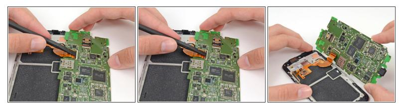
(i) Lay the motherboard down to allow access to the display cable connector.
