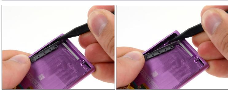
Use the pointed end of a spudger to pry the volume control button assembly away from the edge of the case.
