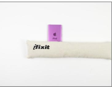
• Lay the iOpener over the plastic tab to loosen the adhesive. Let the bag sit on the device for approximately 90 seconds before attempting to open the panel.
