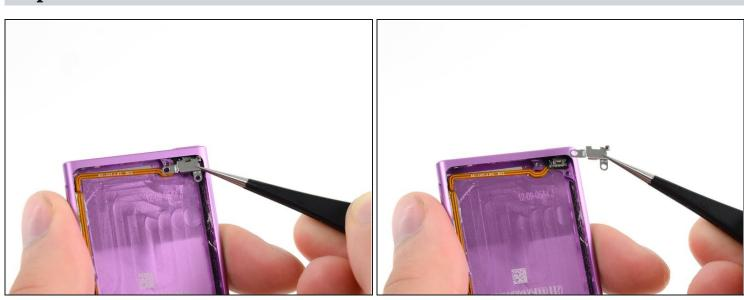
Remove the bracket with a pair of tweezers.
