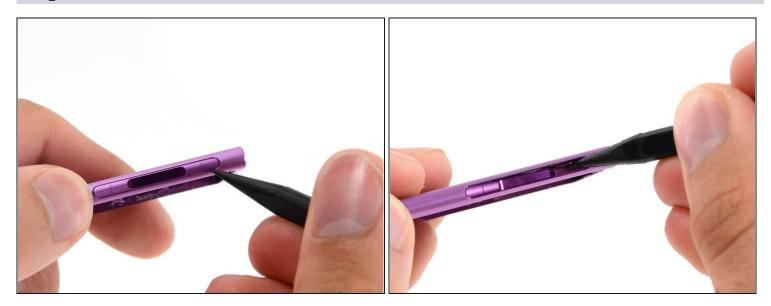
Using a spudger, gently push the volume rocker into the device from the outside.
