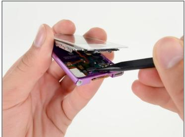
• Use a spudger to release the digitizer cable and display data cable connectors.
