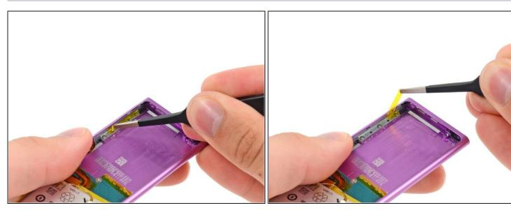
• Peel back and remove any tape covering the volume control button assembly.
