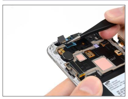
Remove the front-facing camera from the display assembly.
