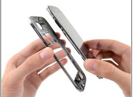
Remove the midframe from the display assembly.
