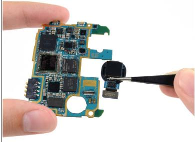
• Using tweezers, or your fingers, slide the rear-facing camera out of its notch in the motherboard.
