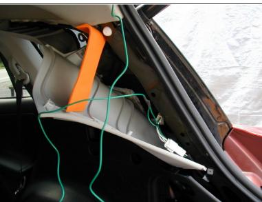
The green wire to the passenger side harness can be run under the top panel which can be pried open slightly along the rubber seal. Run the wire down inside the side panel. Attach to T-connector to the wiring harness.
