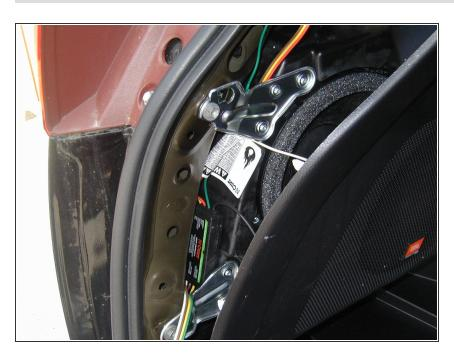
The converter box can be attached to the rear post with the 2-sided tape that came with the kit. By removing one of the bolts of the speaker assembly, the grounding wire can be slid between the assembly and frame and the bolt re-inserted to provide a ground. (If no speaker, a hole exists to insert a hex head bolt)
