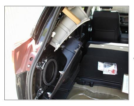
Above the side panels are the rear trim panels that the plastic tools can be pried with one of the plastic tools. The top plastic rivets are tough and may slip out of the panels, but you can pop them out and slide them back on to the panel. Once those are free, you can see the light harnesses on both sides.
