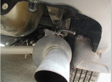
With wiring complete, installing the hitch first required removing the muffler from the rear exhaust isolator, a rubber bracket holding the metal peg attached to the muffler. Some people find this step unnecessary, but working alone, doing this made the installation easier.
