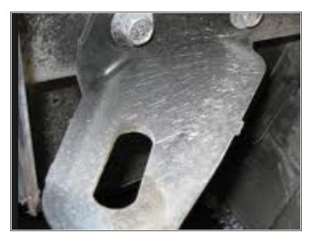
The driver's side has a hidden hitch bracket which needs to be unbolted from the frame before the hitch can be attached. One of those holes will be used and another uncovered to attach that side of the hitch.
