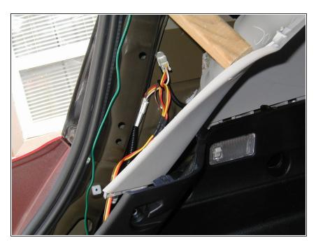
The harness on the driver's side can be separated by pressing the small tab (next step) and reconnected to the red/yellow/brown t-connector coming from the converter.
