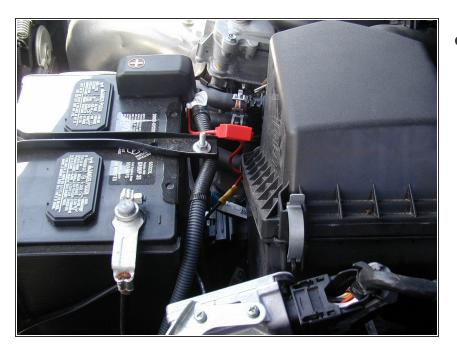
Once in the engine compartment, remove the negative terminal. Attach one of the red fuse link wires to the 12g wire with the remaining straight connector and the other part of the fuse link to the battery positive side using the round connector. Insert the fuse. Re-attach the negative terminal and check with trailer wire tester.
