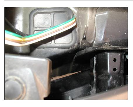
Looking from the underside of the rear metal bumper assembly, I found a rectangular rubber insert which can be removed. The connector to the trailer hitch and wire to the battery can exit the hatch area without any drilling of holes or removing the rubber plugs from the cargo pit. Thread both wires down and through the post connecting the bumper.
