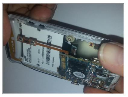
Grasp the sides of the motherboard and gently rock back and forth. This is due to the sticky tape that is on the battery
