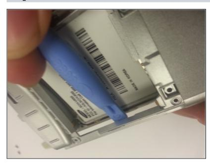
Using the plastic opening tool gently insert it into the seam and work it around till the cover comes off. Being careful of the side buttons that pop off.
