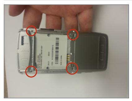
• Unscrew the four corner .4cm Phillips head screws.
