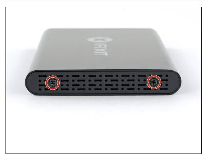
Use the included screwdriver to remove the two Phillips screws.
