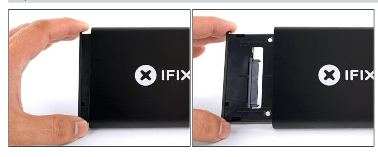
Slide the plastic tray out of the aluminum housing.
