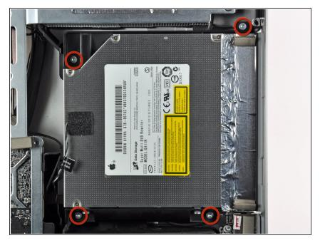
Remove the four T10 Torx screws securing the optical drive to the outer case.
