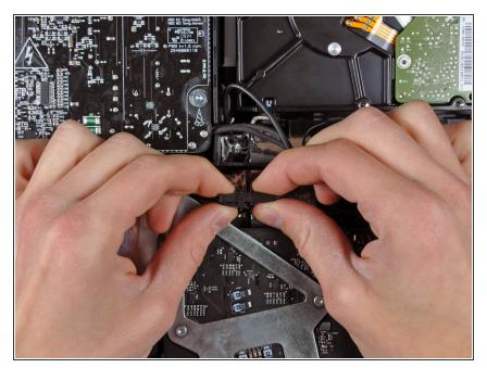
Disconnect the AC power inlet cable by depressing the locking mechanism while pulling the connector away from its socket.
