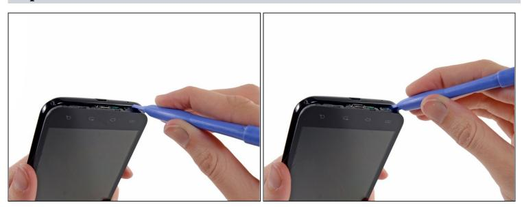
Wedge a plastic opening tool slightly to the right of the micro-USB port, and pry between the midframe and the display to widen the gap.
