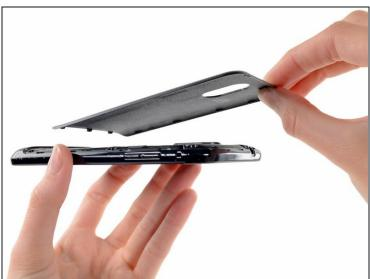
• Lift and remove the rear case.
