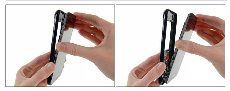
• Pull the micro-USB end of the front panel assembly out and away from the midframe and lift up to free it entirely.
