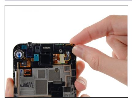
Remove the front-facing camera bracket from the display assembly.
