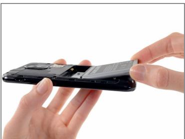
• Lift and remove the battery from the midframe.
