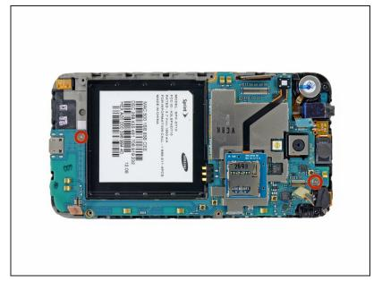
• Remove the two 3 mm Phillips #00 screws.
