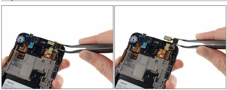
Using a pair of <u>tweezers</u>, or your fingers, remove the front-facing camera/earpiece speaker assembly.
