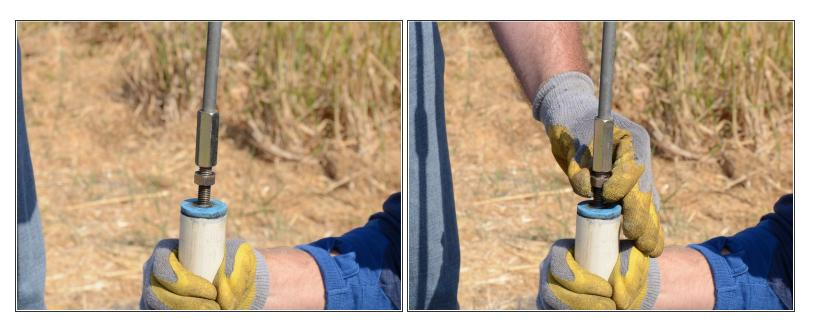
Tighten the jam nut up against the base of the T-handle.
