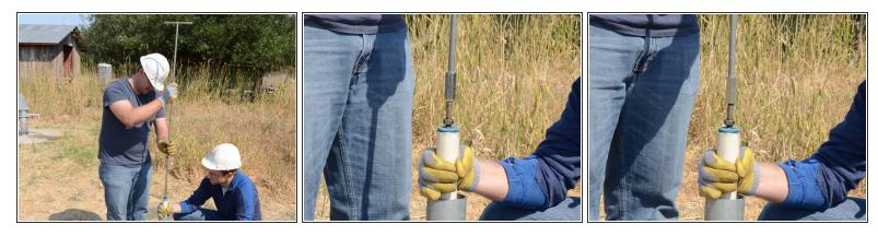
Screw the T-handle onto the top of the riser main.
