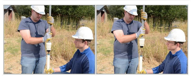
• Lift and remove the handle from the pump. Store the handle in a sanitary place to prevent contamination.
