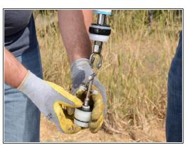
Lift and twist the foot valve to unhook it from the traveling valve.
