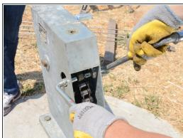
Using the two access holes, place an angled socket wrench on the bolt and nut attaching the chain to the pump handle.
