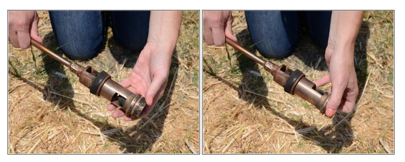
Unscrew the foot valve from the traveling valve.
