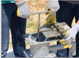
Remove the rod clamp from the tank.
