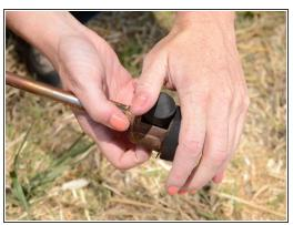
• Use a finger to push the rubber valve poppet out of the traveling valve.
