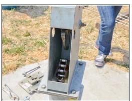
Pull the top of the chain straight off of the pump handle.
