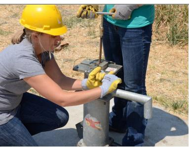
Have one team member lightly pull up on the T-handle, while another loosens the rod clamp. This
