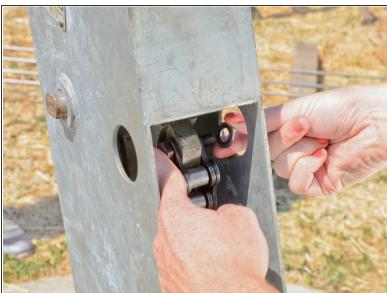
Remove the washer from the chain bolt.
