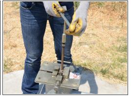
Screw a T-handle onto the top of the pump rod. Tighten the T-handle against the jam nut.
