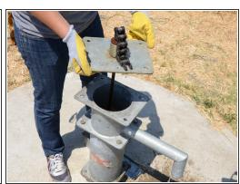
Lift the head flange up about one foot above the tank.
