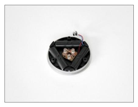
Lift and separate the power switch from the main assembly.
