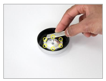
Using a similar technique to that exercised in step 9, slice off the clear plastic extrusions at the indicated positions. These extrusions secure the lens, case and reflector elements.
