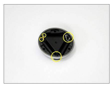
Remove the battery contacts from their mounts, taking care to separate the soldered electrical wires without damaging nearby parts. Note the two smaller contacts which connect to the circuit board.
