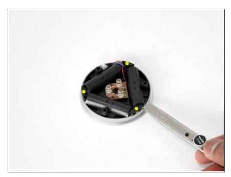
Using the craft knife, prise and loosen the three tabs shown from their mounting points. This will make removing the battery contacts easier in the next step.
