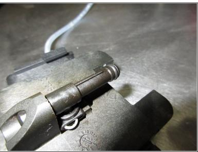
Here you can clearly see how that docking-part works. That seal has big mechanical stress because here the piston docks on.
