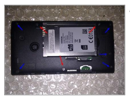
The phone is assembled with eight screws. Using the T4 Torx Screwdriver, remove all eight screws from the back cover. The three small thread screws (red arrows) are fixed on the LCD panel. The four big thread screws (blue arrows) are fixed on the touch screen's frame.
