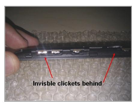
A plastic back plate lies beneath the external back cover. To remove this, place the Plastic Opening Tool between the plastic back plate and the clear plastic tabs on the side of the phone (designated by red arrows). Gently lift up and remove the plastic back plate.
