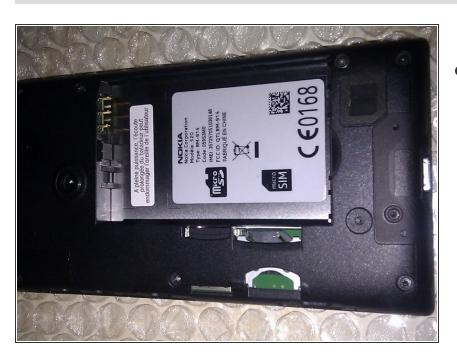
Once the battery is removed, push the SIM card or memory card into its respective slot. The card will then pop out. Remove the card from the phone.
