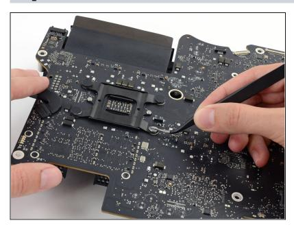
Remove four black stickers from the back of the CPU heat sink.
