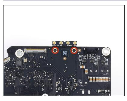
Remove two 3.7 mm T5 screws from the back of the logic board.
