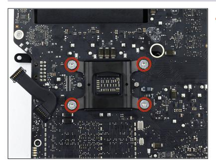
Remove four 12.3 mm T10 screws from the back of the CPU heat sink.
