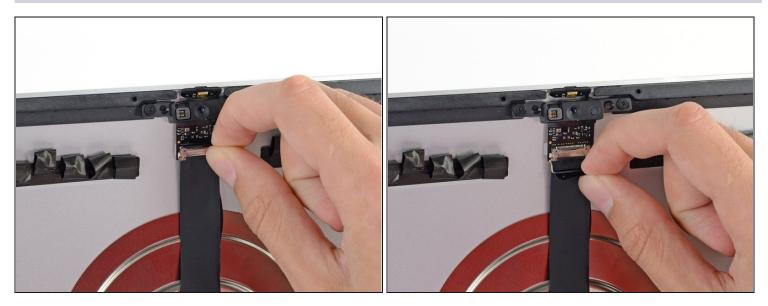
• Flip down the metal retaining bracket on the iSight camera cable.
