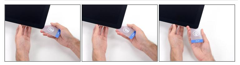
• Insert a second card into the gap between the display and frame in the top left corner.
