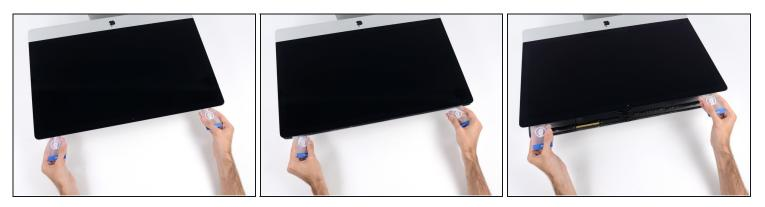
⚠ Only lift the display a few inches—it is still attached to the iMac by data and power cables.
