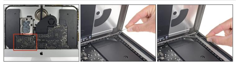
A Be very careful not to touch the capacitor leads or any exposed solder joints on the back of the power supply (boxed in red).
