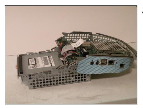
The logic board assembly. This is the heart of the computer, it contains the motherboard, CPU, RAM, V-RAM, PRAM battery, the hard drive, and the optical drive.
