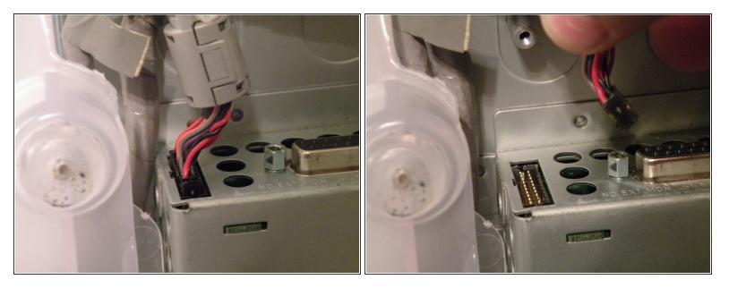
• Remove the front panel connector. (You may also need to remove an additional screw that connects the front panel connector to the logic board assembly).
