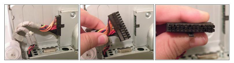
• Remove the power cable from the logic board assembly.
