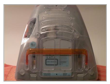
• Start by flipping the iMac upsidedown. It may help to lay it on a towel, so you don't damage the screen, or scratch the face.
