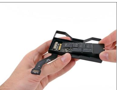
Carefully pull the SSD straight out of its socket on the SSD tray.
