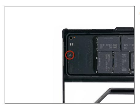
Remove the single 2.9 mm T5 Torx screw securing the SSD to the SSD tray.
