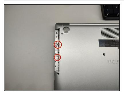
And remove the remaining two screws.
