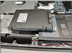
• Now you have access to the inside of the laptop. My device was without an HDD, you can see that its place is empty. You have to remove the metal casing for the HDD, which is held by these screws. There are four screws provided with which you can fixthe HDD to its place (in my case a 2,5 inch SSD) on the metal frame.
