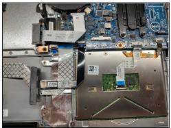
• The SATA cable was under the cable for the USB and card reader module and I had to remove my battery to switch those cables because I couldn't put the SSD correctly in place. The battery is fixed with 4 screws. Make sure you disconnect it before you start to remove.
