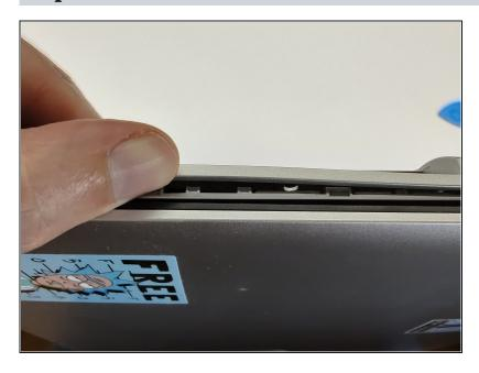
Now you can start removing the plastic case, with the help of the opening tool and the spudger. Be gentle, but also ferm, this should come off fairly easy. If you don't have an opening tool, make sure that the tool what you will use is made from a softer material than the case of the laptop.
