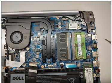
• The device has two slots for memory, it is very easy to upgrade. You just have to pop in the new RAM in the empty slot.
