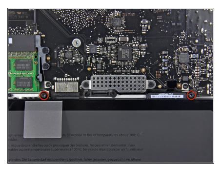
Remove the two exposed five-point Pentalobe screws along the top edge of the battery.
