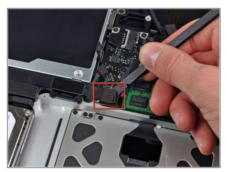
Use the flat end of a spudger to pry the hard drive/IR sensor cable connector up off the logic board.
