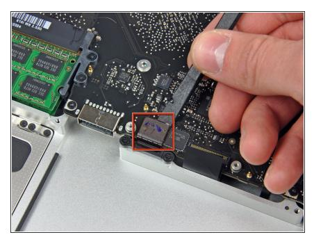
Use a spudger to pry the trackpad flex ribbon cable connector up off the logic board.
