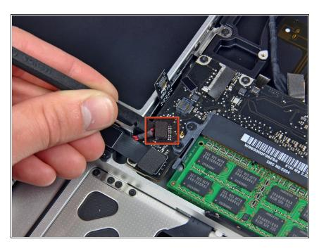
Using the flat end of a spudger, pry the subwoofer connector straight up off the logic board.
