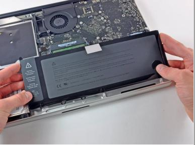
• Lift the battery by its plastic pull tab and slide it away from the long edge of the upper case.
