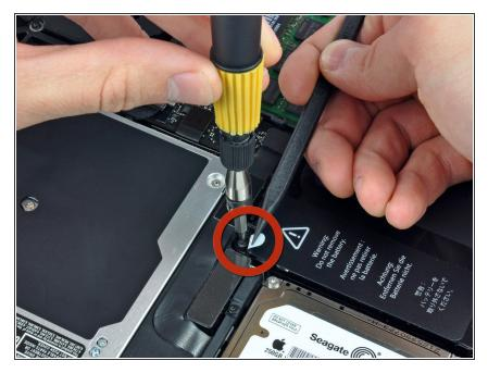
Use the tip of a spudger to bend back the finger of the "Warning: Do not remove the battery" sticker while you remove the five-point Pentalobe screw hidden underneath.
