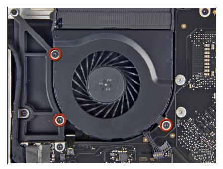
Remove the three identical T6 Torx screws securing the fan to the upper case.
