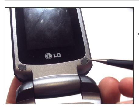
Use tweezers to remove the two rubber covers found at the left and right corners below the inside screen.
