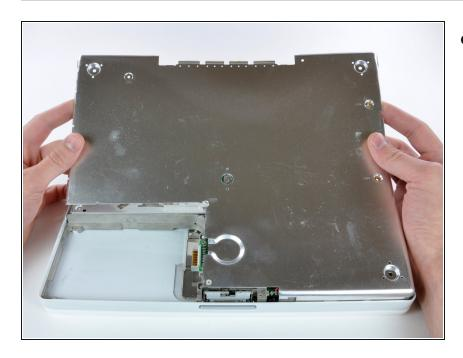
• Lift the bottom shield off.
