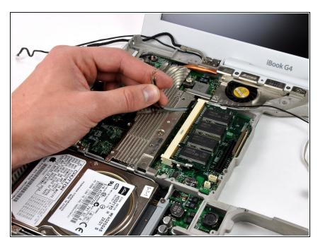
De-route the AirPort antenna cables from the heat sink.
