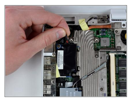
Disconnect the RJ-11 cable from the top of the modem.
