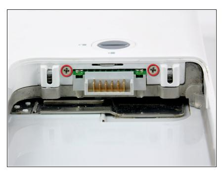
Remove the two 4.5 mm Phillips screws on either sides of the battery contacts.
