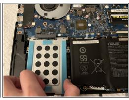
♠ Do not lift the HDD up, as you may damage the connector highlighted in red.
