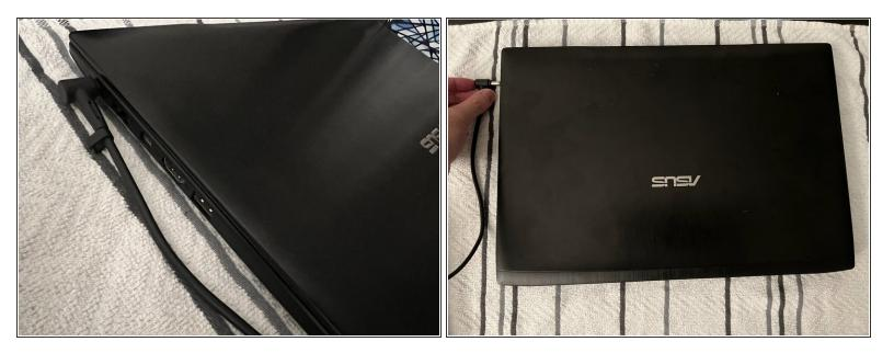
Before disassembling the laptop, turn the laptop off and make sure it's unplugged from the power supply.
