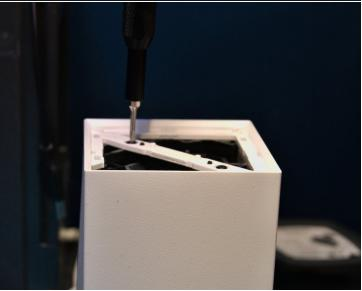
Use a <u>Torx T6 screwdriver</u> to unscrew the two screws that were previously hidden under the top cover.
