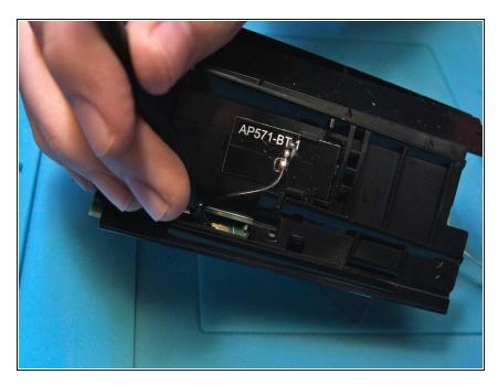
Unclip the Bluetooth antenna, the same procedure as the WiFi antennas.
