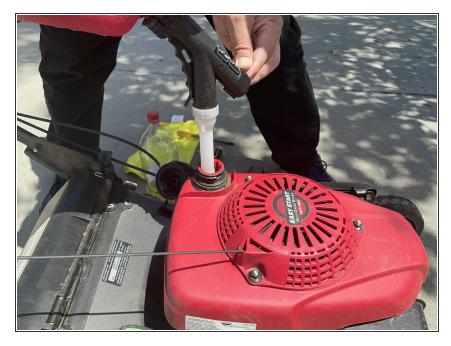
Use the fuel can to refill the lawnmower now that the contaminated fuel has been removed.
