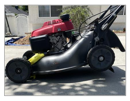
Tilt the lawnmower forward so any remaining fluids can make their way out.
