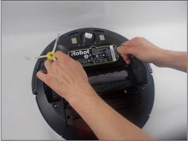
• Remove the battery by pulling directly up on the grey pull tabs.
