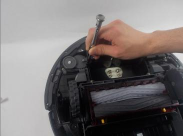
• On the underside of the Roomba, use a Phillips #1 screwdriver to remove the three 15.5 mm screws.
