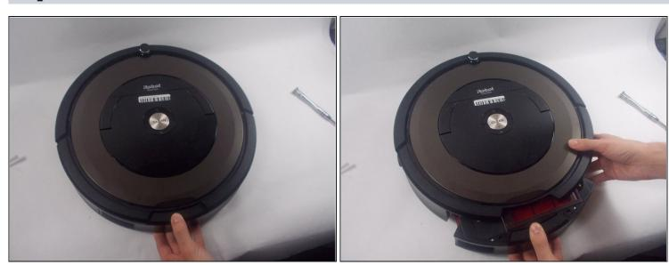
• Remove the collection bin by pressing the release button on the top side of the Roomba and pulling straight out.
