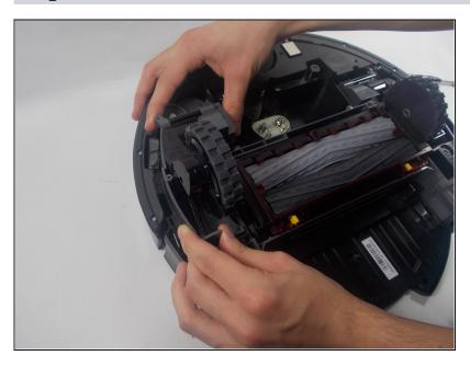
Grip both sides of the casing and pull it straight out.
