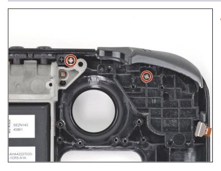
Use a Phillips driver to remove the two 5.2 mm screws securing the left bumper assembly.
