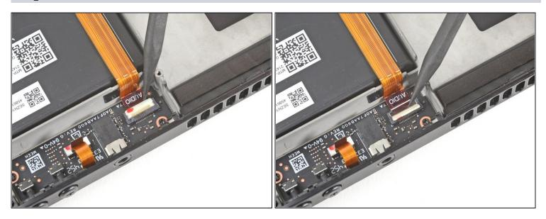
• Use the pointed end of a spudger to lift up the small locking flap on the audio cable's ZIF connector.
