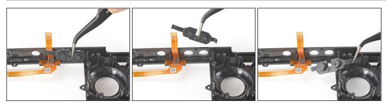
• Use a pair of tweezers to remove the volume buttons by pulling them up and away from the front shell.
