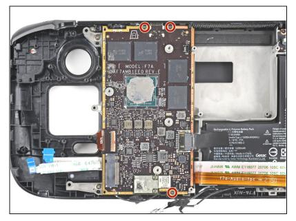
• Use a Phillips driver to remove the three 3.7 mm screws securing the motherboard.
