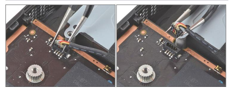
• Use a pair of tweezers to grip the edges of the fan connector and pull up to disconnect it from the motherboard.
