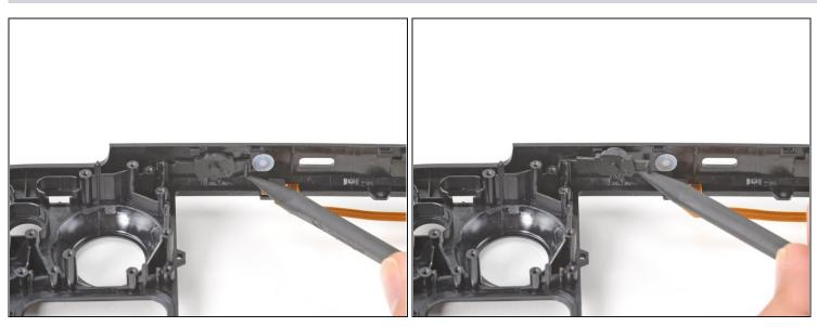
• Use the pointed end of a spudger to lift the rubber flap to the right of the power button up and out of its plastic clip.
