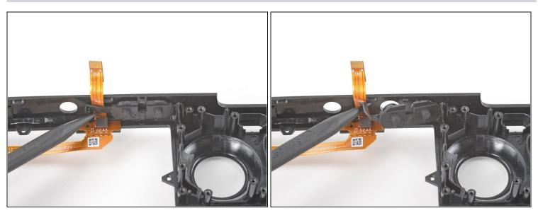
• Use the pointed end of a spudger to lift the rubber flap to the left of the volume buttons up and out of its plastic clip.
