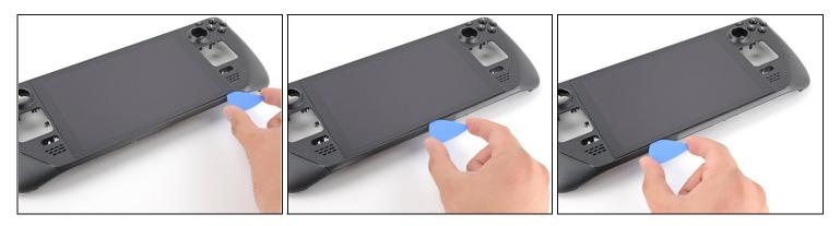
• Slide the opening pick across the bottom edge to slice the adhesive.
