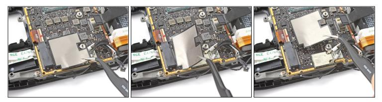
• Use a pair of tweezers to peel up and remove the Wi-Fi shield tape.
