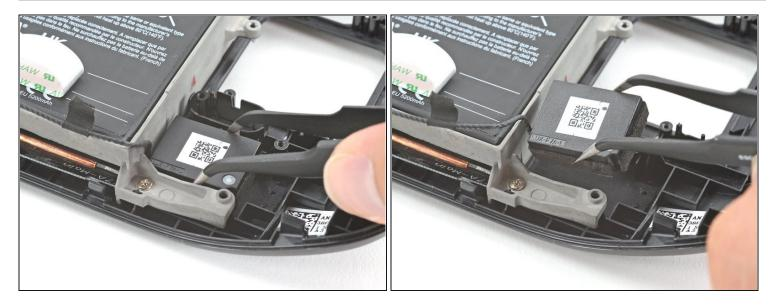
• Use a pair of tweezers to grip and remove the left speaker from its cavity.
