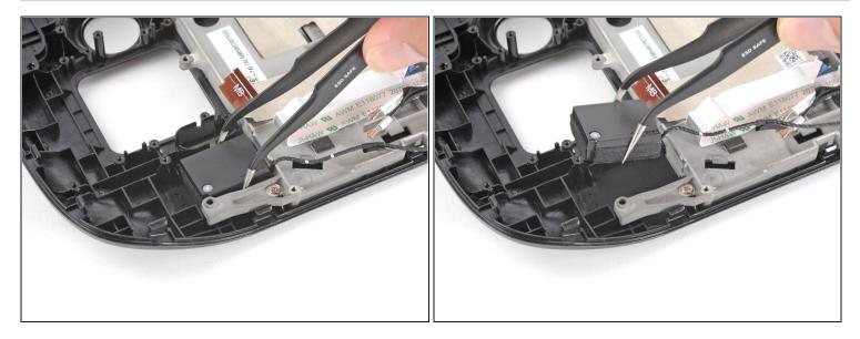
• Use a pair of tweezers to grip and remove the right speaker from its cavity.
