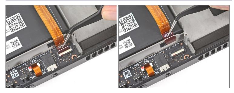
Use a pair of tweezers to slide the cable out of its connector.
