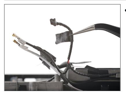
Use a pair of tweezers to peel up the tape bundling the speaker wire to the Wi-Fi antenna cables.
