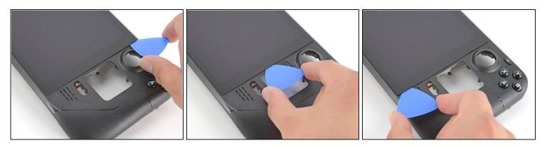
• Slide the opening pick down the right edge to slice the adhesive.
