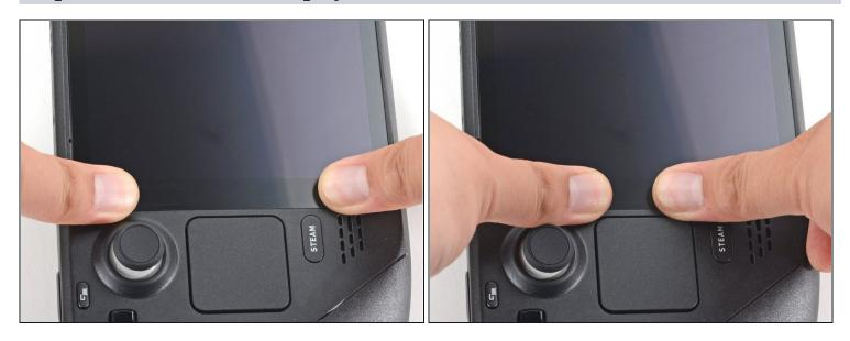
• Set the new display in place on the midframe and press firmly along the edges for 20-30 seconds to ensure a good adhesive bond.
