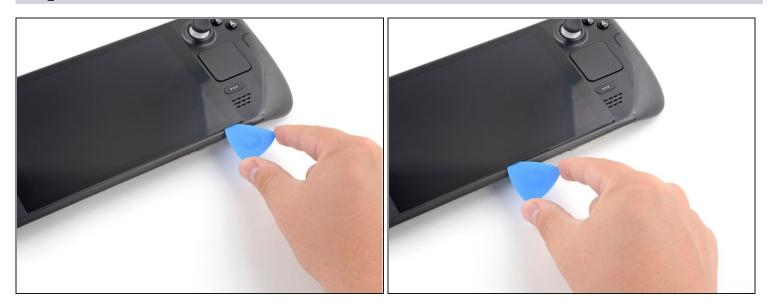
• Slide the opening pick across the bottom edge to slice the adhesive.
