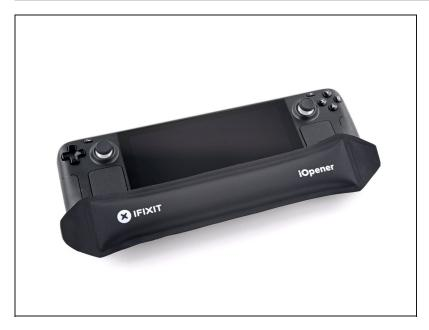
• Heat the bottom edge of the display for one minute.
