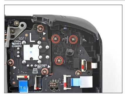
Use a Phillips driver to remove the three 5.2 mm screws securing the left trigger bracket.
