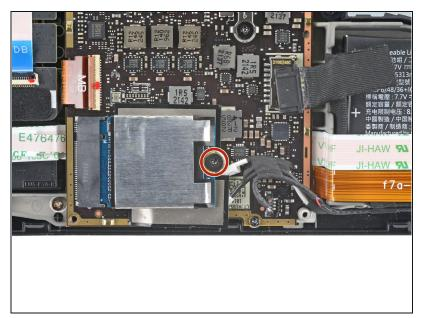
Use a Phillips driver to remove the 3.4 mm screw securing the SSD.
