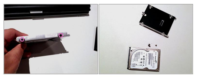
To remove the hard drive from the bracket remove the two M3.0×4.0 screws from each side of the hard drive.
