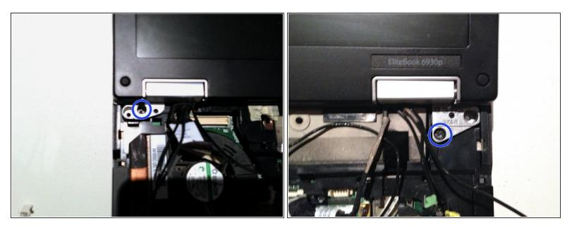
The display assembly will be unsupported when the following screws are removed. To prevent damage support the display before removing the screws.
