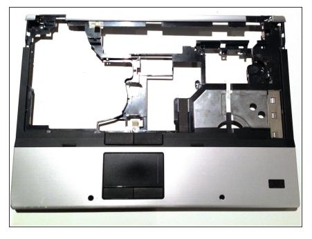
• Lift the rear edge of the top cover until it separates from the base of the laptop and lifting it straight up.
