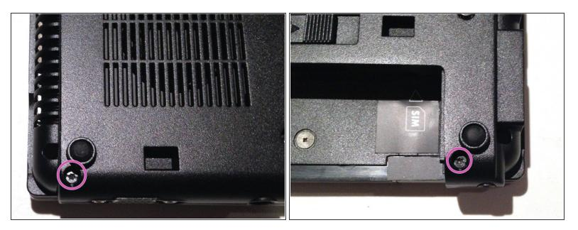
• With the laptop upside down, locate and remove the two Torx T8 2.5×7.0 screws.
