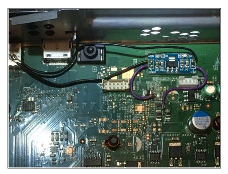
The soldering was as follows: From mobo L3B1 (north side) 5v, in to converter Input. From converter Output 3.3v, in to L5A1 (east side). From converter ground in and ground out (both) to the housing of the analog a/v module.
