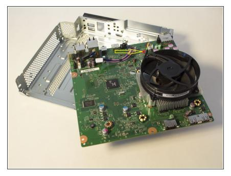
Open the console, remove the hdd/dvd caddy, unplug (but no need to remove) fan. Locate mosfet at U5A1.
