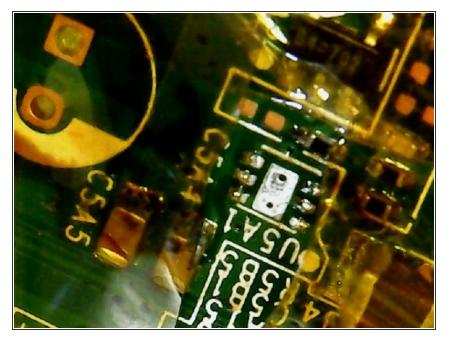
Flux it, hot air (medium low air pressure), remove. I found that I had to crank my hot air station to 375 degrees, at lower temps it just wasn't budging.
