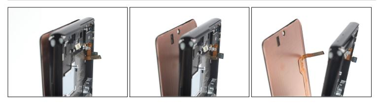
• Carefully thread the fingerprint flex cable through the gap in the midframe.
