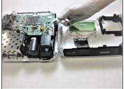
Gently disconnect the white ribbon cable connecting the motherboard to the button panel.
