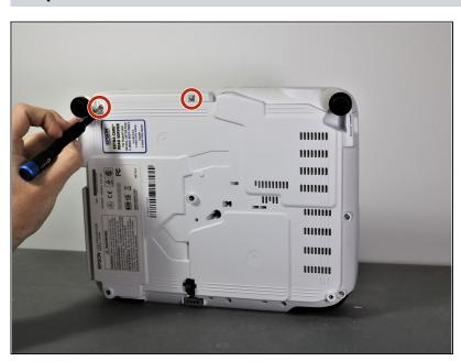
Use a Phillips #1 screwdriver to remove the two 10 mm silver screws from the bottom of the device.
