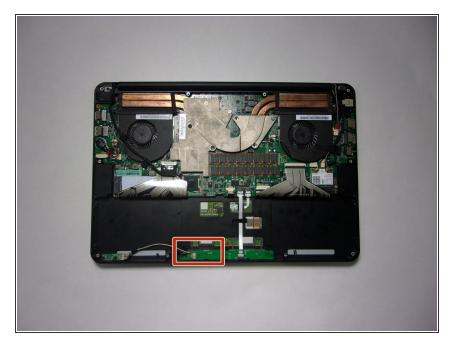
• Detach the battery's ribbon cable from the motherboard.
