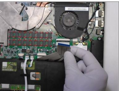
Flip up the black plastic lock-bar on the <u>ZIF</u> connector, then gently pull the ribbon cable directly out
