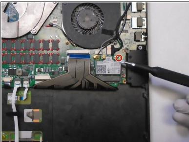
Use a Phillips #0 screwdriver to remove the single 3 mm screw from the upper-right corner of the Wi-Fi card.
