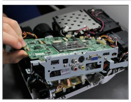
Lift and remove the motherboard up and away from the device.
