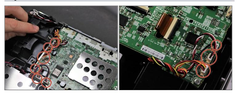
• Using a spudger or a plastic opening tool, disconnect all of the wires connected to the motherboard.
