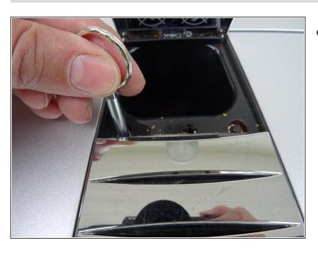
Also remove the two oval head screws underneath the ground coffee compartment lid.
