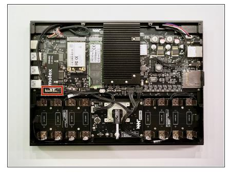
Unplug the UI1 (keyboard) and UI2 (trackball or trackpad) cables from the motherboard.
