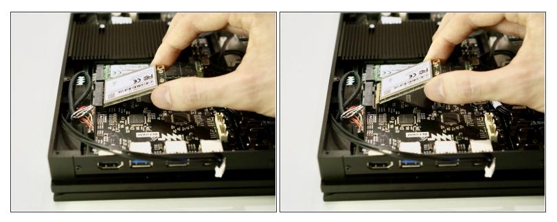
• Pull the WiFi card out of its mPCIe socket on the motherboard.
