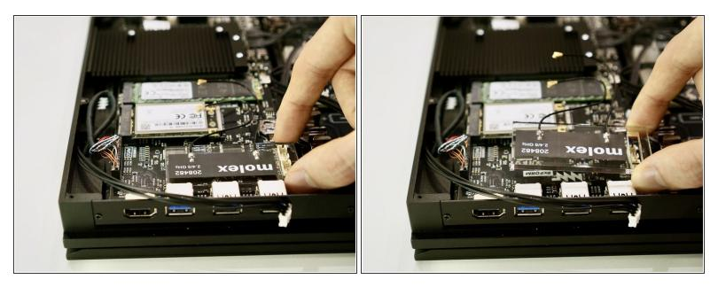
• Lift the acrylic holder with the Molex MIMO antenna out and set it aside.
