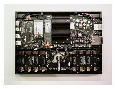
Remove the single M2×4 pan head screw securing the SSD to the motherboard.
