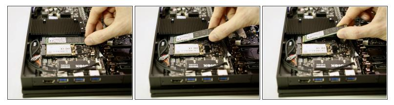
Lift the free end of the SSD up slightly and pull the SSD straight out of its M.2 socket on the motherboard.
