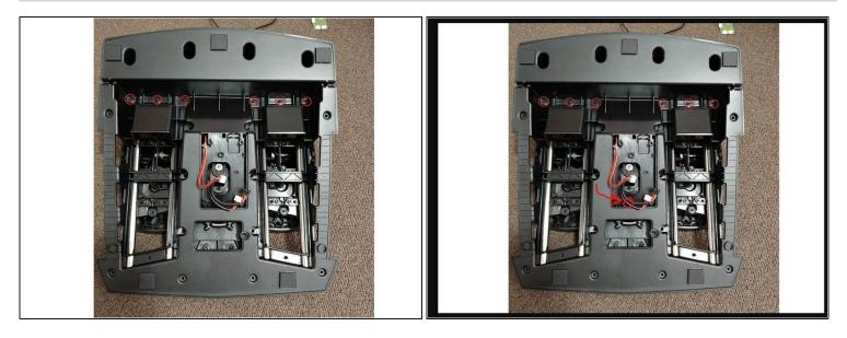
• Remove the six screws in the top recess.
