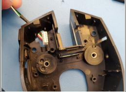
hold the mouse in one hand and use your index finger to push down on the rubber connector (shown)
