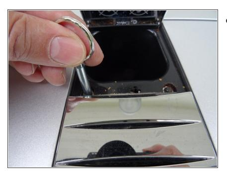
Also remove the two oval head screws underneath the ground coffee compartment lid.
