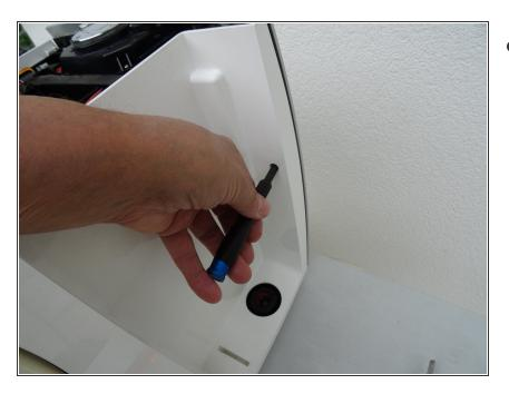
Remove the Torx T15 screw on the side panel with the water tank.
