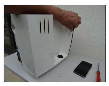
• Pull the left side panel slightly towards the back and remove it.
